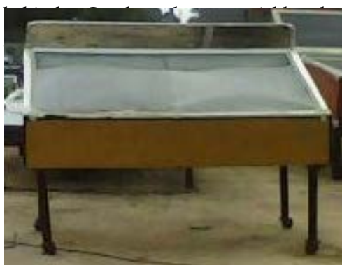
Fig. 1: Rectangular-shaped solar still
